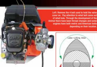
The easiest way to find when the valves are closed is to feel for the compression stroke. This is done by removing the spark plug and putting your thumb completely over the hole and sealing it off. By turning the engine over slowly by hand in a clockwise rotation (when looking at the flywheel), you can feel the engine start to make compression and feel air leak past your finger. Stop turning the engine at this point.
