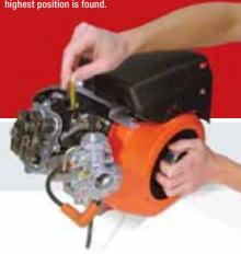
by hand. What this does is slightly lift the valve on the compression stroke to relieve some of the pressure so it can be turned over easily. This release then swings out of the way when the engine reaches operating speed. The lash can't be set on this compression release or the setting will be dramatically wrong. By setting the lash a little past TDC you eliminate the possibility of running into this.
