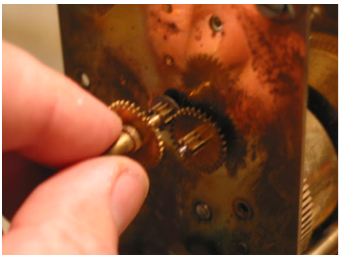
Illustration 7: First the hour wheel comes off.
