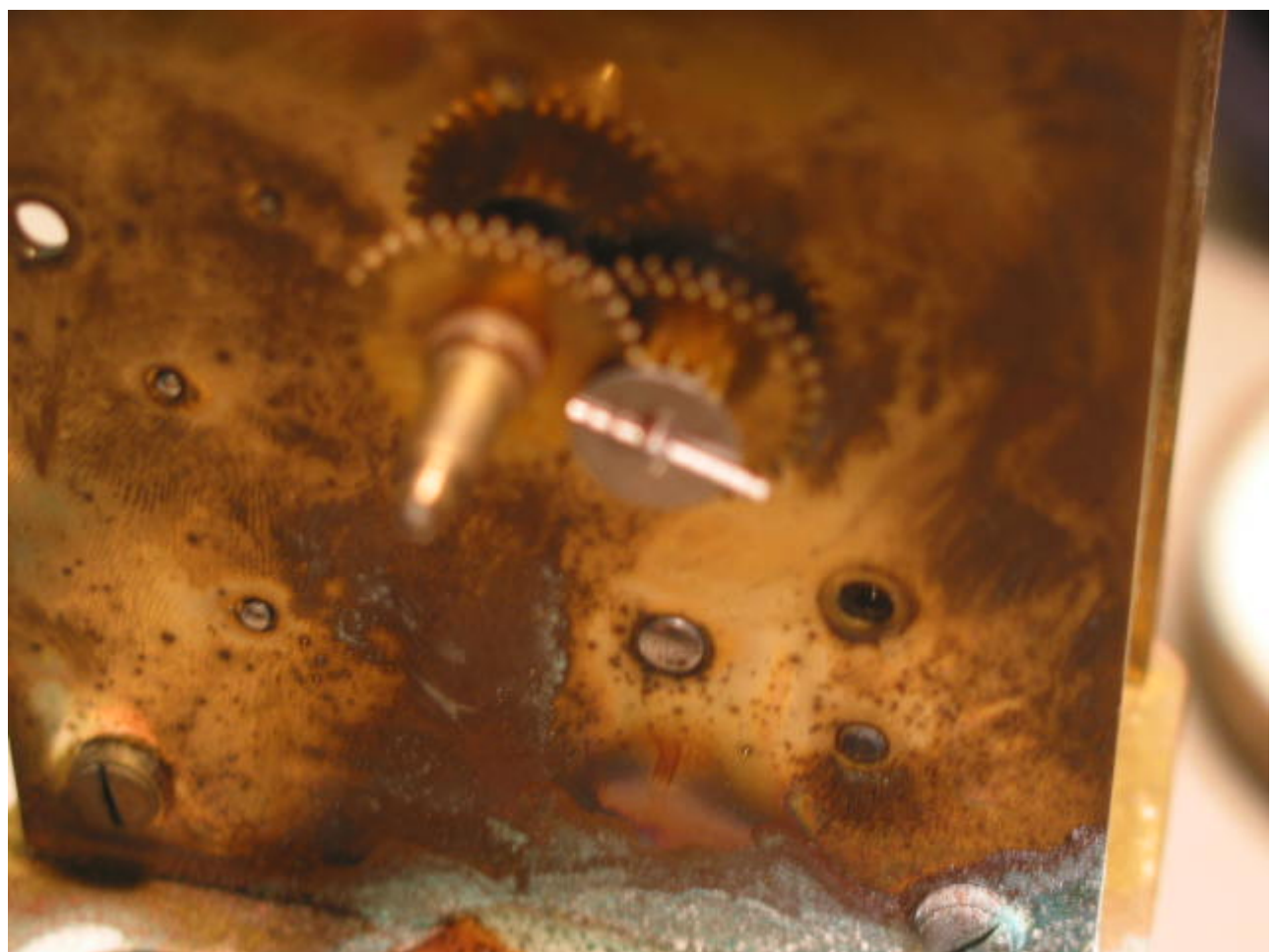
Illustration 5: The whole assembly is held on by a pin and steel shim, I'll take this off.
