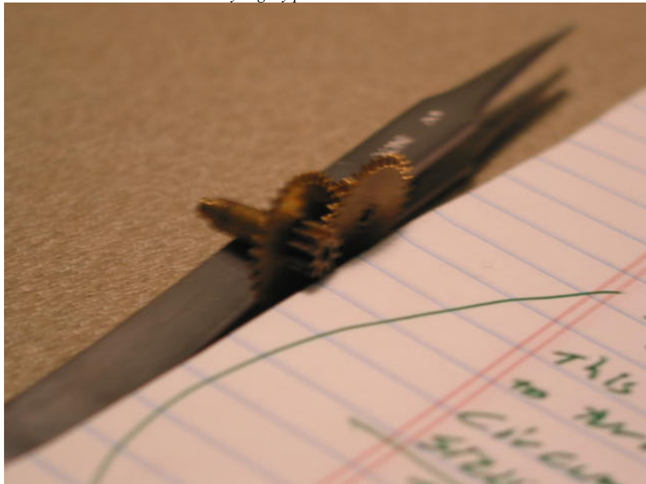
Illustration 14: So that is the equivalent of a 1 to 12 difference in circumference. This is also a good design because the reduction wheel reverses the direction back to clockwise for the hour wheel.
