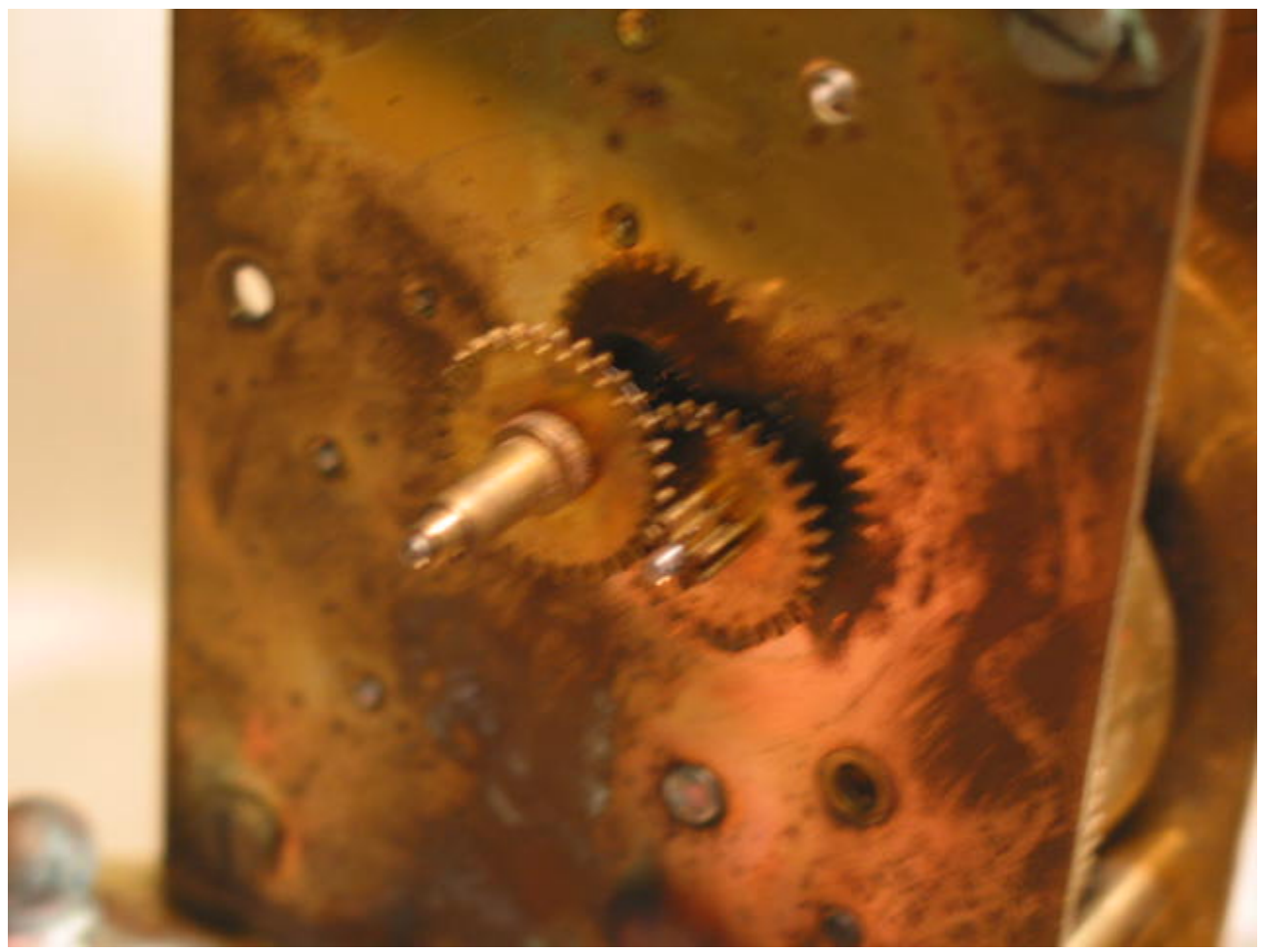
Illustration 6: Now I am free to take the wheels (gears) off.
